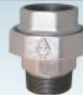
Whole Union, M&F, conical joint, iron to iron seat
